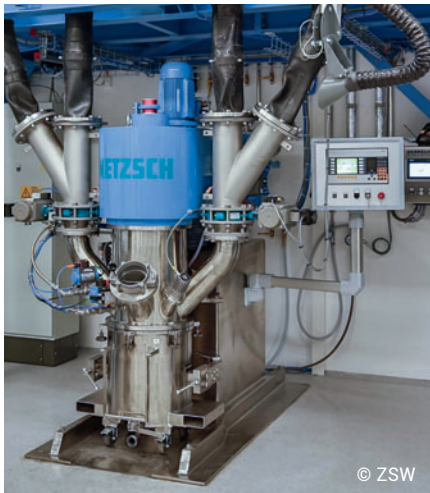
Production research at the ZSW: 60-litre mixing system for electrode pastes. Image: ZSW
