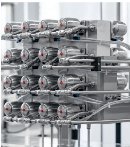
Electrolyte filling of the battery cells with GEMÜ multi-port valve block in stainless steel
