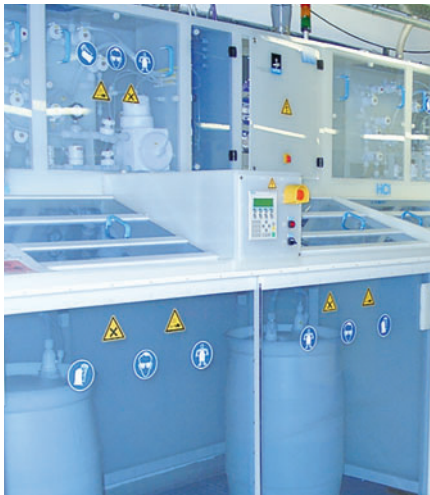
Chemical supply module for chip production
