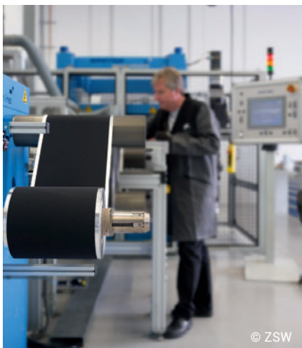
Production of electrode strips under near series conditions at the Centre for Solar Energy and Hydrogen Research (ZSW). Image: ZSW
