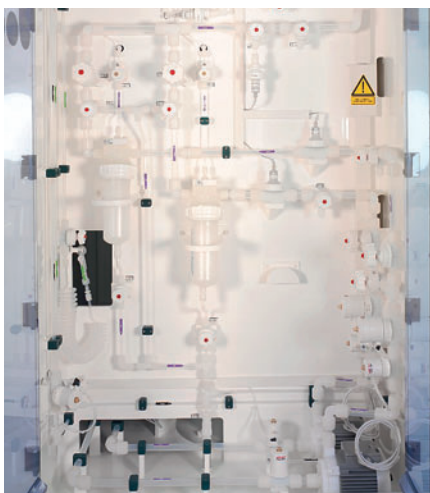
Supply module for technical chemicals
